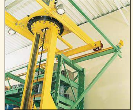
4 ft Cantilever Overhang
