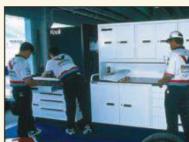
Using modular cabinets outfitted with a combination of drawers, doors, and casters, several state-of-the-art mobile workstations were built for the Valvoline race team.
