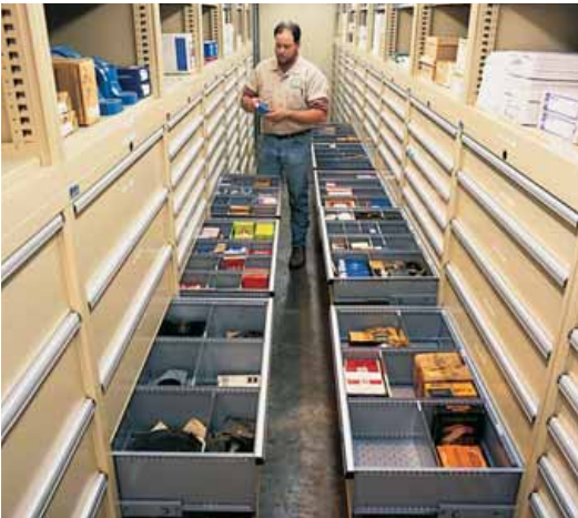
Stacked HS shelf and drawer cabinets allow narrow aisles.
